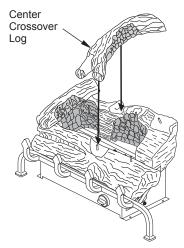
Figure 19 - Installing Center Crossover Log (VYS18 Series Shown)
